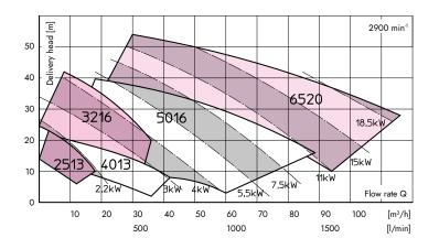
The quick suctioning immersion pumps type SZ are ideal for pumping liquids with high air inclusions such as emulsions, grinding and cutting oils. The impeller of the SZ is a combination of an open impeller and a compressor impeller, which allows the simultaneous transport of air and media with pollutants. This makes the SZ pump the ideal quick suction-
