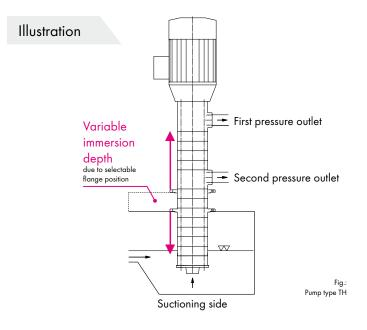
Multistage immersion pumps type TH are characterized by variable immersion depths due to selectable flange positions. They are ideal for pumping clean or slightly polluted fluids such as lubricants, alkaline solutions, acids and solvents used in washing, clean-
