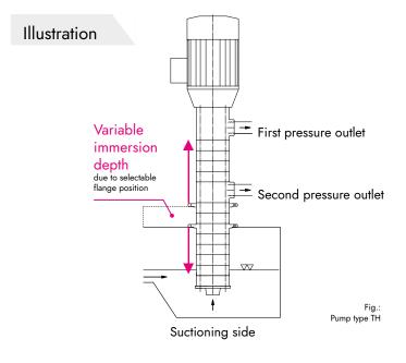
Multistage immersion pumps type TH are characterized by variable immersion depths due to selectable flange positions. They are ideal for pumping clean or slightly polluted fluids such as lubricants, alkaline solutions, acids and
